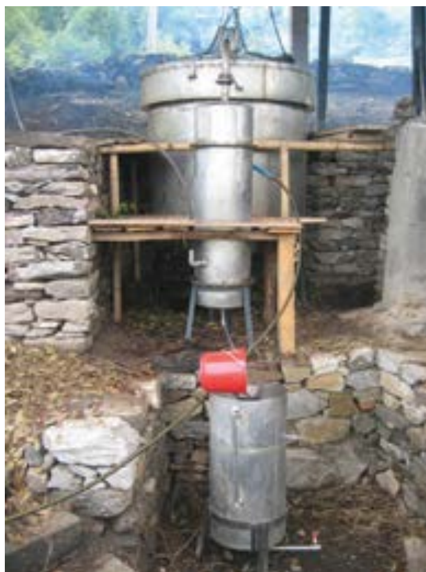
A unit for distilling essential oils in Dolakha district, Nepal
