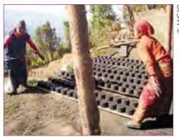
Women pressing the char mixture into the moulds to produce the briquettes, which are then left to dry in the sun
